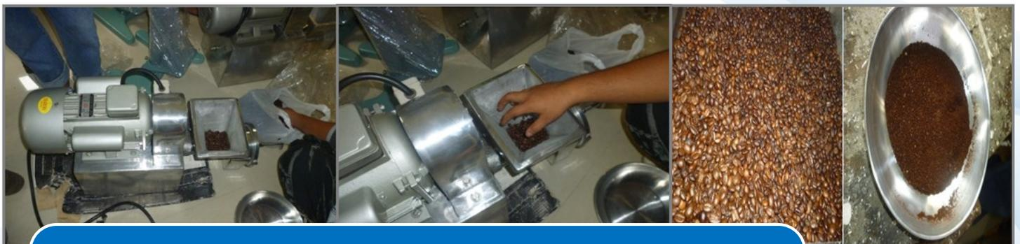
Coffee Grinder - equipment used for grinding all kinds of beans and grains either wet or dry like coffee, rice, corn, mungo, paminta, ube or cacao. This equipment is operated by 2 hp motor, 220 volts, single phase 60 Hz with a capacity of 60 kg/hr. The units were distributed to three DA stations for demonstration purposes.
