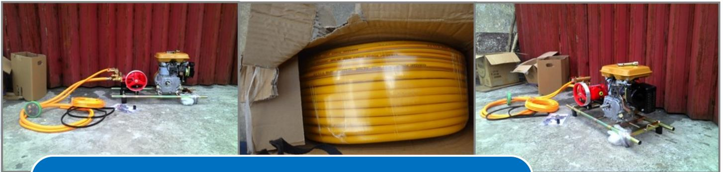
There were 25 units of power sprayer distributed to support the enhancement of off-season mango production in the region. The unit is powered by 5 hp gasoline engine with 100 m high pressure hose, 2.5-3.0 megapascal (Mpa) capacity with 8.5mm diameter. These were distributed to mango growers association and DA stations in the region.
