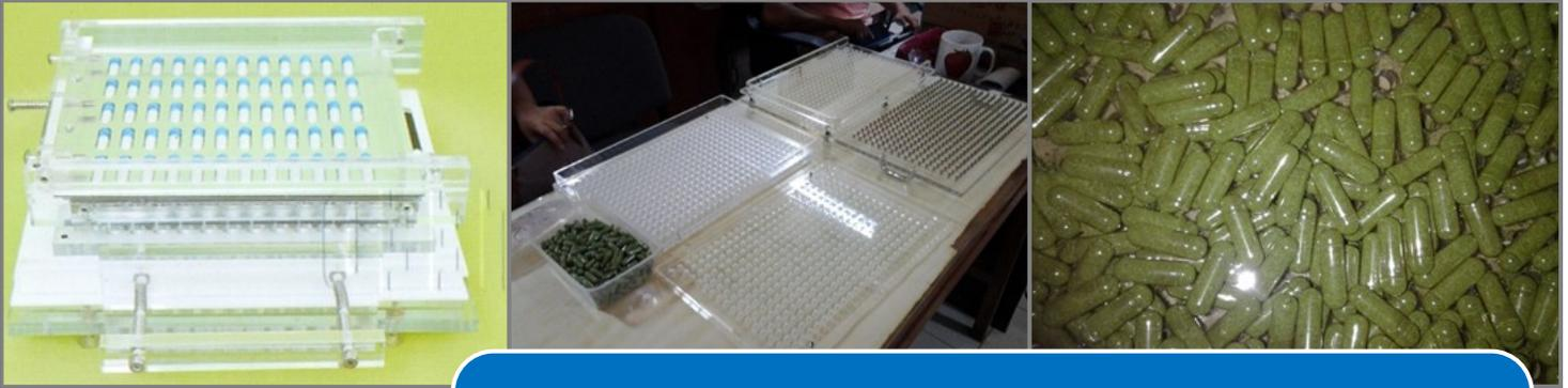
The equipment is used in the production of vegetable capsules for food supplement. This is a manually operated capsule filling machine with 400 holes per operation. Procured three units of this machine and distributed to three DA stations for demonstration purposes.
